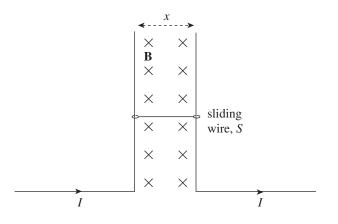
The mass of the sliding wire, S, is m. If the sliding wire S crosses a region that contains a uniform magnetic field **B**, how much current must be carried by the wire to keep S from sliding down (due to its weight)?
